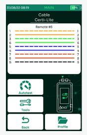
Figure 5 - Wiremap with Remote ID#8 Identified
