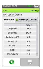
TestPro's LiveWiremap™ facilitates rapid cable continuity testing with automatic display of result the moment the cable is attached. TestPro offers fault location for Return Loss and NEXT aiding in problem identification. Support for MPTL, Patch Cord, Cat8, and Coax is available through hot swappable Adapters. At the completion of the Autotest, you will get a highly visible Pass or Fail indication, and test results can be automatically saved with a customizable labeling scheme.
