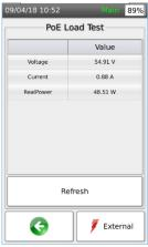
For those pesky intermittent power issues, TestPro allows for sustained loading of the PSE over longer periods, through external loads. This allows you to monitor live for any power fluctuation that drops below the required level threshold. TestPro can also characterize the cabling links for DC resistance unbalance parameters either as part of a standard cable certification Autotest or as a one-off quick test.
