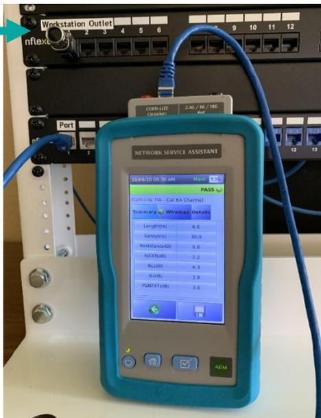
The main test unit of NSA is similar to a main unit of AEM's award-winning certification tester, TestPro that comes in a pair for dual-ended testing. Because the NSA performs a single-ended cable test, it comes with a small passive termination plug called *NSA Remote*, at the remote end, which helps to significantly reduce the overall cost of the test equipment while providing an ANSI/TIA 1152-A compliant cable test.
